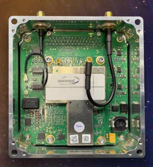
Spaceopal's HAUT-S is an onboard real-time orbit determination and time synchronization (ODTS) component for low Earth orbit (LEO) and low-middle Earth orbit (MEO) satellites, delivering decimeter-level orbit accuracy and nanosecond-level time synchronization for a wide range of space missions with anti-spoofing (OS NMA) and interference mitigation for enhanced resilience.
